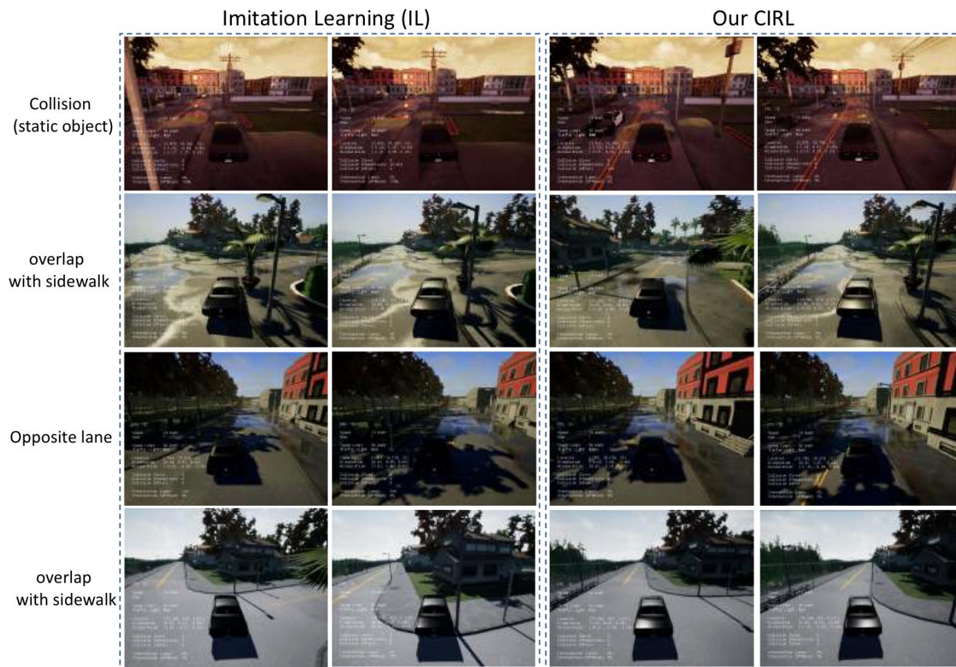
Fig. 7. Visualization comparisons between the imitation learning baseline [15] and our CIRL model. We illustrate some driving cases for straight and one-turn tasks, and show the IL baseline fails with some types of infractions (e.g. collision with static object, more than 30% overlap with Sidewalk, in opposite lane) while our CIRL successfully completes the goal-oriented tasks. For each case, two consecutive frames are shown.
